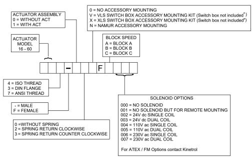
\* VLS and XLS switch boxes MUST be ordered as a separate item with comment assemble items 1 and 2 together
