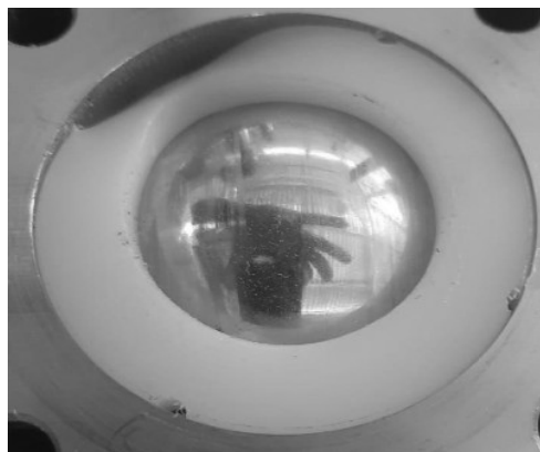
Figure 6: Distorted valve seat due to incorrect closure position
