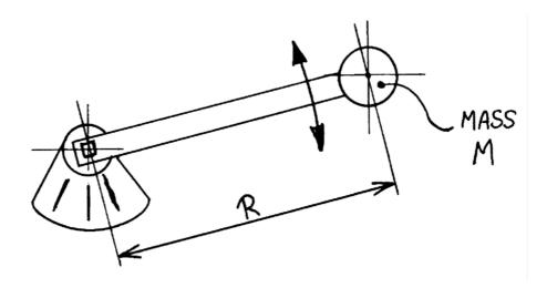
Time for 90° travel = T (sec.) Moment of Inertia = I (kg m<sup>2</sup>) (for a mass M (kg) at radius R (m):  $I = MR^2$ )
