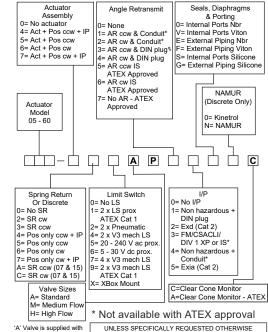
'A' Valve is supplied with all sizes up to and inc' 09 'M' Valve is supplied with 10-15 'H' Valve is supplied with sizes 16-60 Recommended spring unit for model 14 actuator is 4900 type. This should be coded 12 49AP or 13 49AP instead of the usual 12 AP or 13 AP. The same applies to other specially
