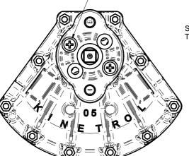
Screw positions shown for 03 mounting -Tighten to 5Nm (45 lbf in)
