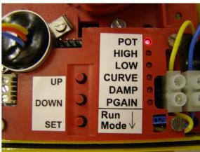
1.12 - For clockwise units rotate the potentiometer anti-clockwise about quarter of a turn until the POT LED flashes.
