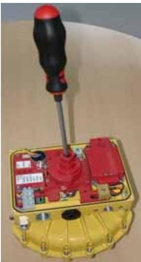
Lift out the carrier plate with the shaft.
