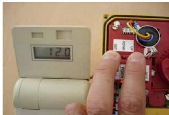
1.2– Disconnect air pressure, remove the lid and connect signal above 4mA.
