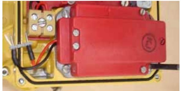
The complete unit can now be tested with 4-20mA signal.
