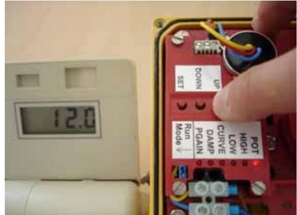
Press the SET and UP buttons: the LED flashes while the actuator's vane moves toward its 100% end stop. When its movement is stopped by the physical end stop, the positioner waits briefly, then moves the actuator steadily downscale until it runs against the bottom physical end stop, where again it waits briefly, and finally moves quickly back to the original position.
