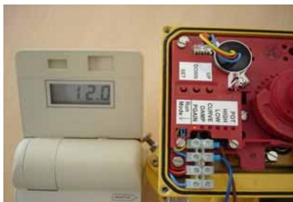
If not, check the signal input and its polarity. If the LED fails to light, the circuit may have to be replaced (spare part = SP1007).
