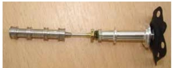
Clean the valve liner sleeve (in situ in the servo valve block) and the bobbin valve, using plenty of ethanol. Clean out the air channels as far as they are visible.
