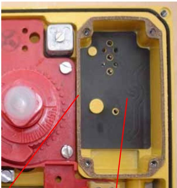
Top cork gasket      Servo valve base gasket
