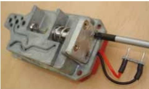
Replace the complete servo valve in its recess in the positioner body, taking care that the cork gasket under the servo valve rim is in place, fit the 4 screws with Loctite, screw them all down finger tight, and then tighten them down hard.
