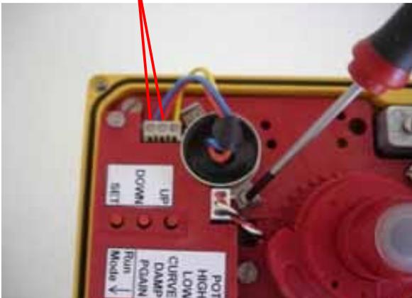
Rotate the potentiometer slowly until the 'POT' LED flashes. Re-tighten the clamp screws. Now the set-up mode can be left by pressing DOWN button until each LED is off.
