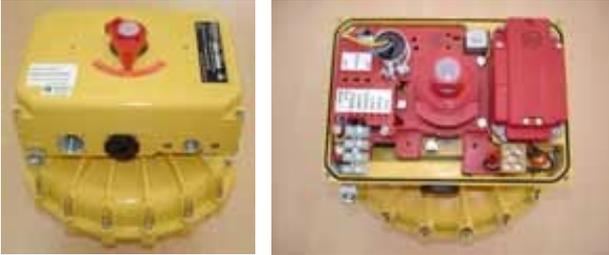
Undo the 5 screws securing the carrier plate assembly and remove the white plug from top of the shaft.
