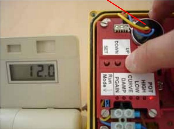
If the 'POT' LED flashes it means that the feedback potentiometer is set correctly – go to section 1.6
