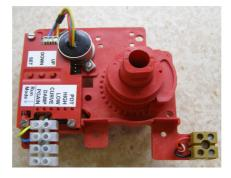
1.6 With the circuit has been removed, it is advisable to mark the position of positioner shaft with a permanent marker to ensure the shaft remains in the same position.
